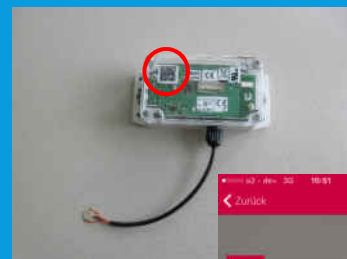
Micro controller radio sensor with QR Code – direct link to dashboard
